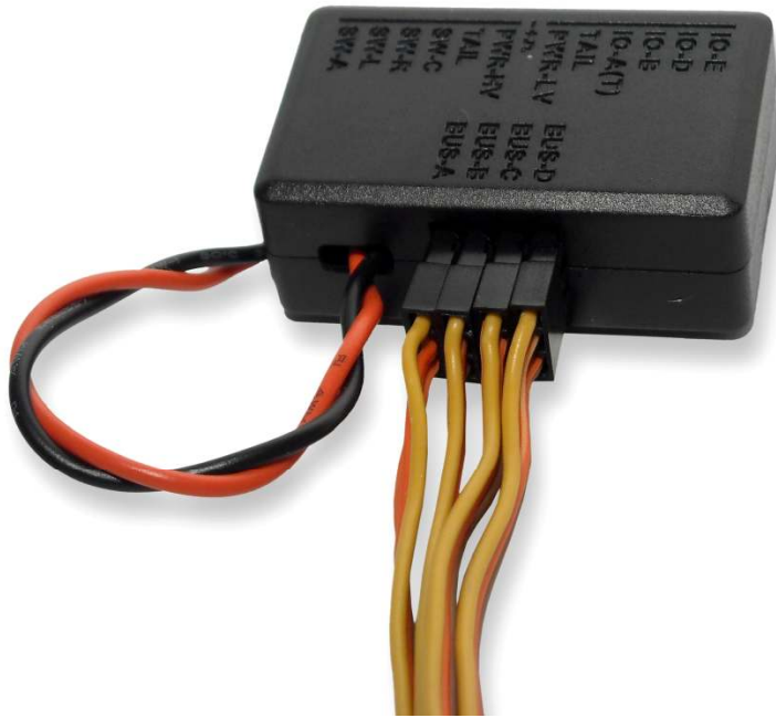
Figure 6.2 – SK-PW7 Signal Bus Connections
