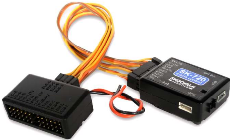
Figure 6.5 – SK720 Connections to SK-PW7
