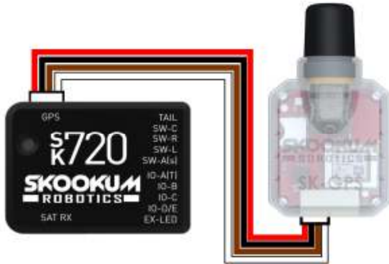
Figure 5 - Connecting the SK-GPS to the SK-720
